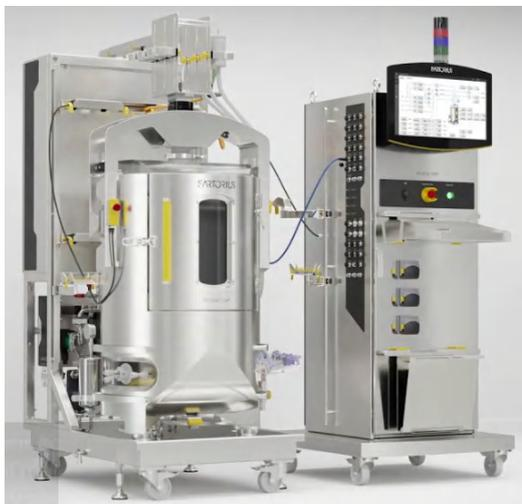
Zollner supplies the Control Tower for operation and control and the energy supply unit, named the Supply Box, for the Biostat STR<sup>®</sup> Generation 3 from Sartorius AG used for vaccine production.
